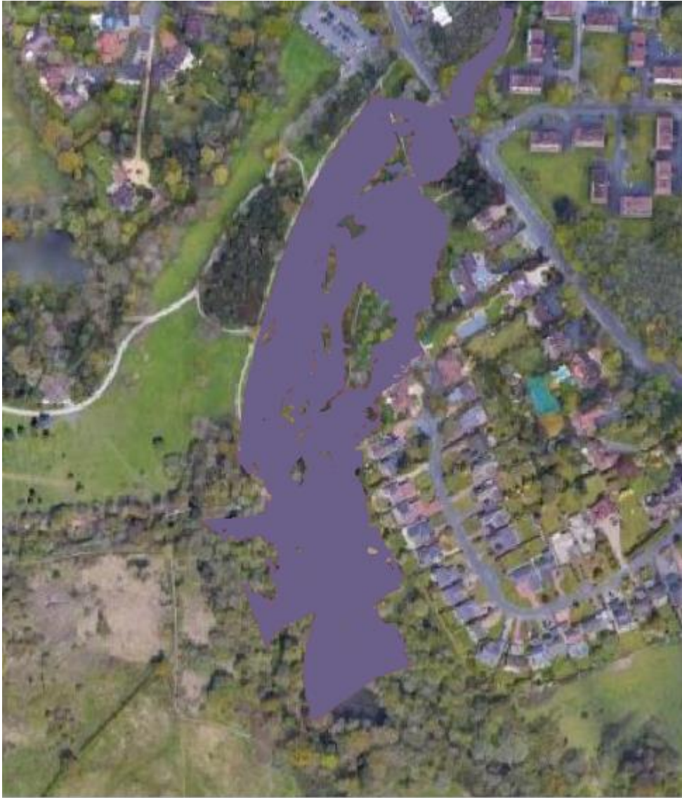
Figure 3.18. 1 in 20yr flood extent change, blue = baseline, red = restored (where red is visible indicates flood extent increase, purple indicates no change and blue indicates reduction in flood extent).
