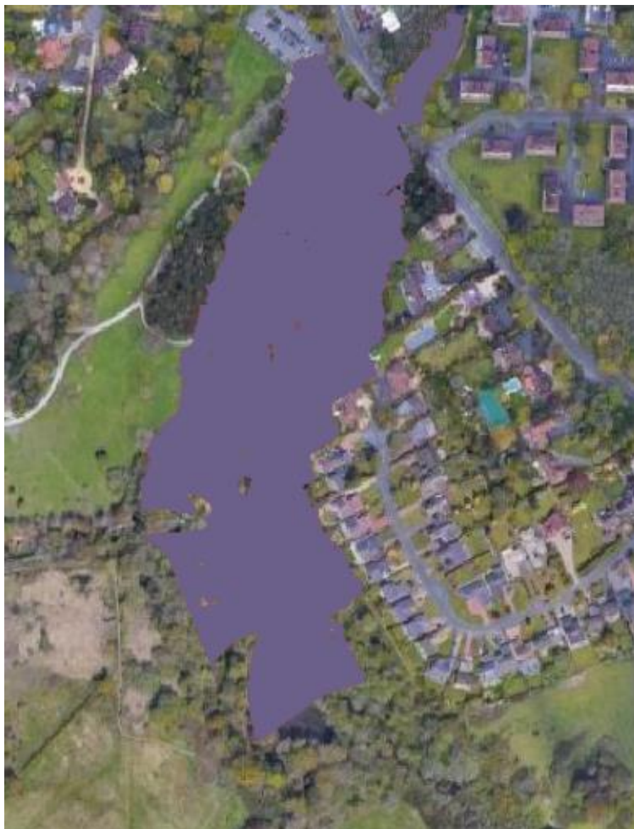
Figure 3.17. 1 in 100yrCC flood extent change, blue = baseline, red = restored (where red is visible indicates flood extent increase, purple indicates no change and blue indicates reduction in flood extent).
